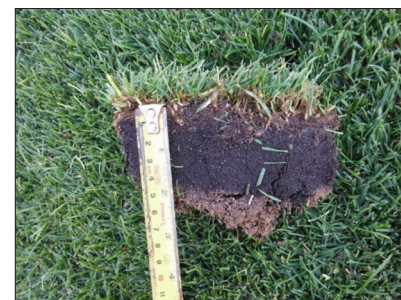
Fig 37. Poor-draining soil-based turf placed over free-draining root zone – will not perform well under heavy rainfall.
