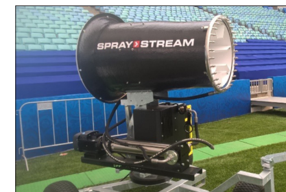
Fig. 11. Examples of pitch side ventilation and cooling fans used to manage turf health
