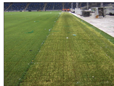
Fig. 85. Warm-season turf on which panels (see Fig. 86) were left in place for three days (left) and five days (right).
