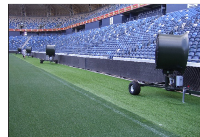
Fig. 11. Examples of pitch side ventilation and cooling fans used to manage turf health
